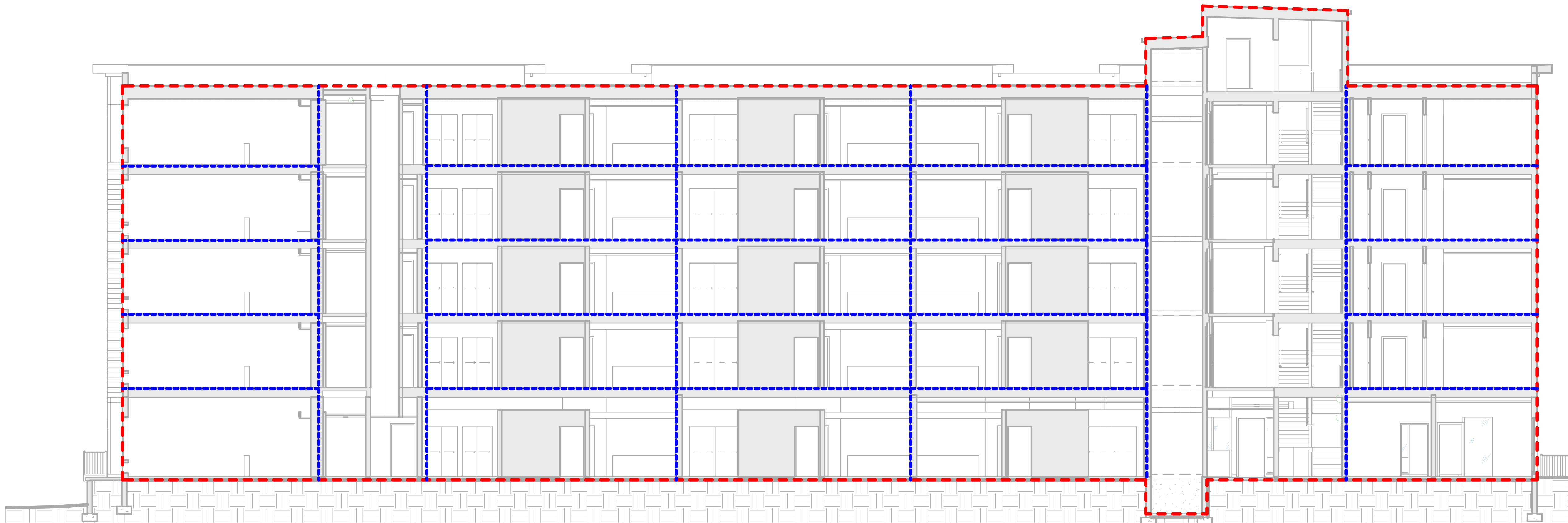
16 SECTION AIR BARRIER DIAGRAM
